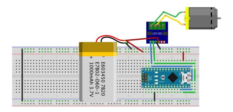
A simple sketch showing some of the behavior that is possible using the L9110S is available here.
