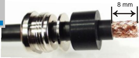
Remove 8 mm of the PVC sheath from the end of the cable with a knife.
