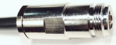
Slide the prepared cable end into the connector housing until stop. Tighten smoothly with two wrenches 16 mm so that there is still a small gap visible between the nut and the connector housing.
