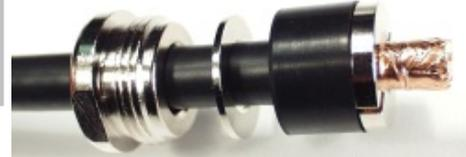
Bend copper braid at 90 degrees to cable body. Push in contact ferrule between copper foil and braid until stop. Trim braid even to rim of ferrule. Slide rubber gasket down to the contact ferrule.
