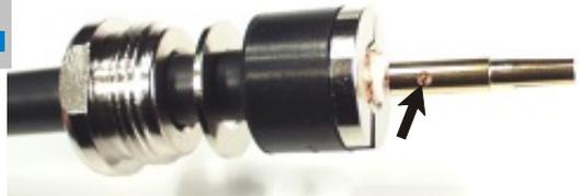
Slide center pin cautiously on center conductor and solder carefully through the little hole..
