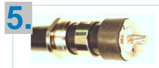
Remove foil and dielectric with a knife. The center conductor must remain absolutely round, if necessary bend carefully.
