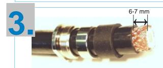
Remove 6...7 mm of the PVC sheath with a knife.
