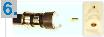
Push center pin in teflon isolator. Then put center pin cautiously on center conductor Hint: Before attaching the center pin a very thin vaseline film may be applied to the center conductor. This improves the intermodulation attenuation and prevents corrosion.
