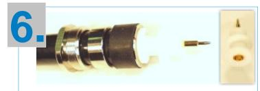
Push center pin in teflon isolator. Then put center pin cautiously on center conductor. Hint: Before attaching the center pin a very thin vaseline film may be applied to the center conductor. This improves the intermodulation attenuation and prevents corrosion.
